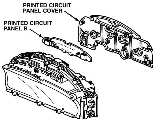
3. Reconnect the electrical connectors to the gauge assembly. Position the assembly so you can get at the back.
