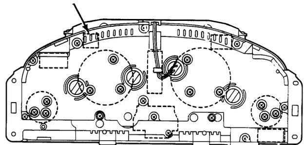
8. Reinstall printed circuit panel B and the printed circuit panel cover.
