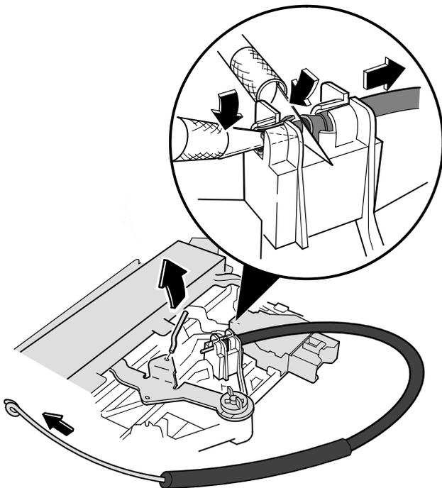
3. Slide the large section of the cable housing out of the cable holder, being careful not to damage the cable stoppers.
