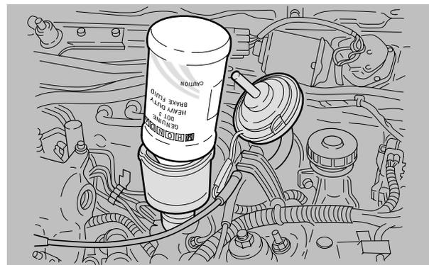
**Pressure Bleeding:** Install the pressure bleeder. Using the bleeding sequence in the appropriate S/M, bleed at each caliper until the fluid is clear. (Follow the pressure bleeder instructions.)
