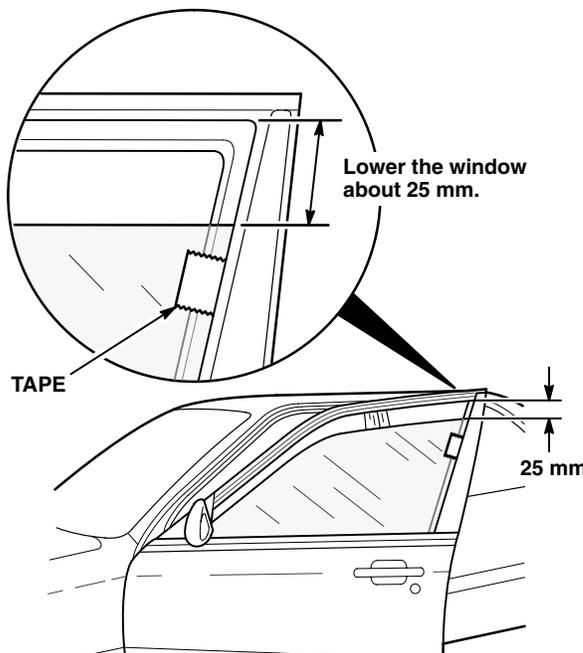
2. Raise the glass fully. Measure the gap between the tape and the run channel lip.
