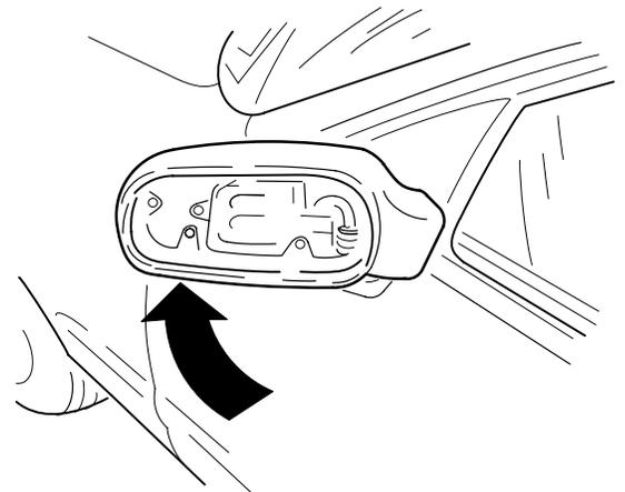
5. Remove the five screws that attach the bezel to the mirror housing. Pry the outer edge of the bezel away from the housing to release the clips on the pivot end.
