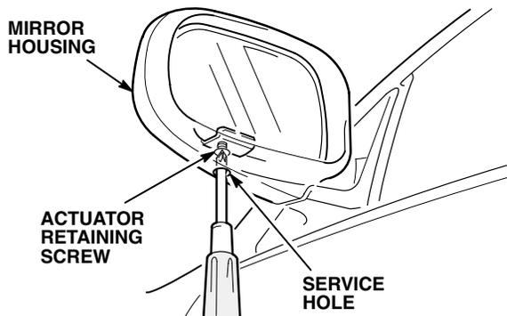
3. Remove the actuator and the mirror holder assembly from the mirror housing; then, disconnect the connector.
