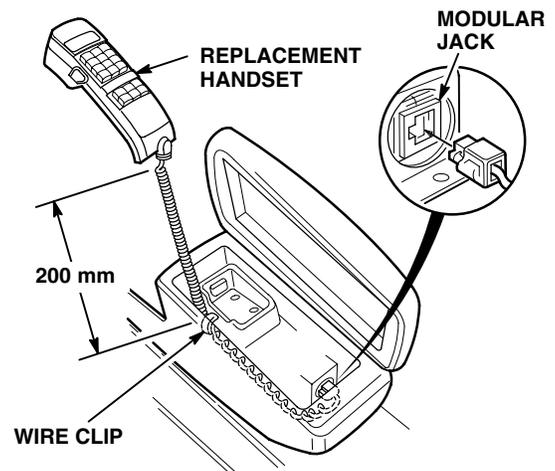
6. Set the handset in the cradle; then, remove it and bring it to your ear several times. The cord should lie flat and not interfere with the back of the console.
