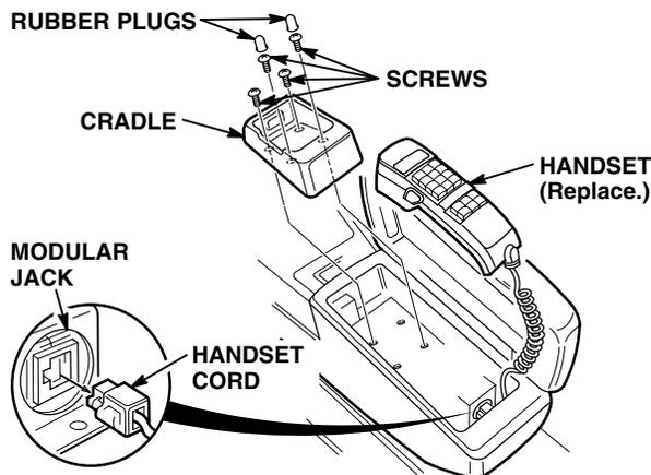
2. Remove the cradle from the console bracket (two rubber plugs, four screws).
