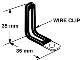
4. Reinstall the cradle with the bent wire clip under the front mounting screw on the driver's side. Tighten all the screws securely, and install the two rubber plugs.
