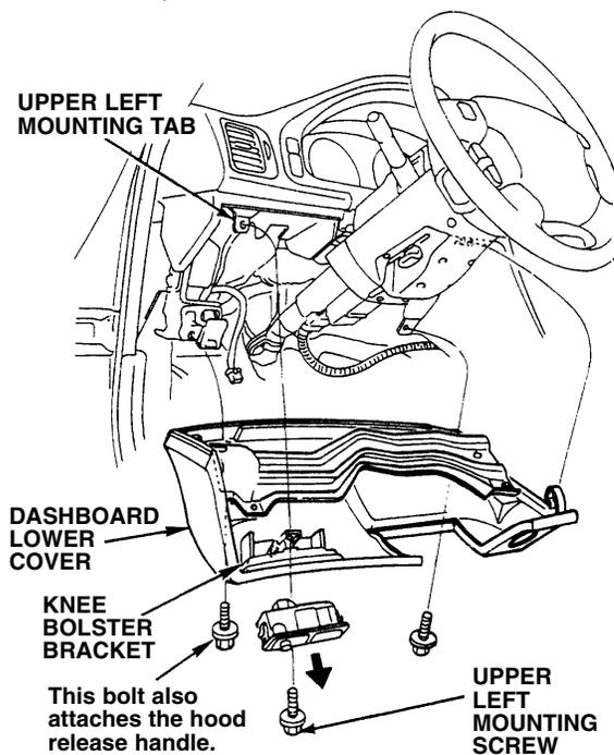
2. Remove the three lower dashboard cover mounting screws, then remove the cover.
