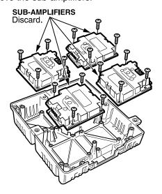
6. Make sure the amplifier box is facing as shown. Each replacement sub-amplifier has a white dot or a black dot to show if it is for the front or the rear speakers. Install the sub-amplifiers with a white dot on the left side of the box. Install the sub-amplifiers with a black dot on the right side.
