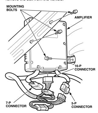
3. Remove the 10 mounting screws from the cover of the amplifier box. Remove the cover. These screws have a 1/4" hex head. If you have only metric wrenches, use the handle of a removable-blade screwdriver. This should have a 1/4" hex.
