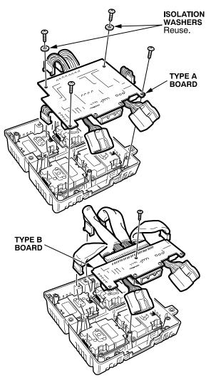
5. Disconnect the electrical connectors from the four sub-amplifiers. Remove the mounting screws, and remove the sub-amplifiers.
